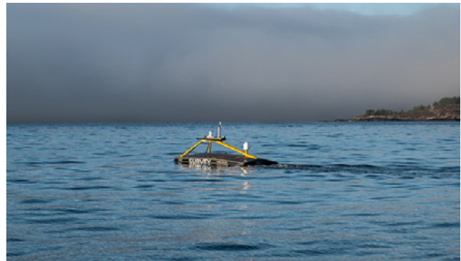
The X-07 vessel collected data from the Ormen Lange gas field in Norway, while remotely operated by experts based in Ireland.
